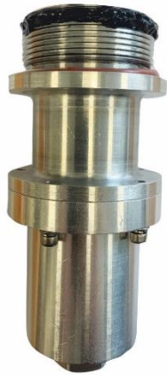
Figure 5-8: Bushing Adaptor with initial threads covered in grease
