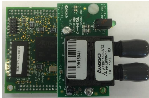
Figure 5-23: Fibre optic module
